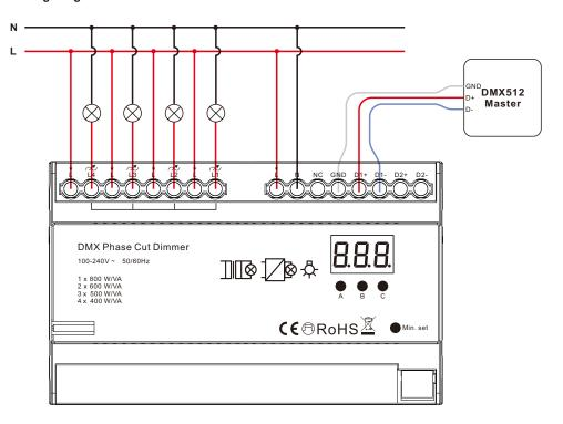
This phase dimmer adopts trailing edge dimming (reverse phase control), the dimming range is 1%~100%, please make sure the connected loads support reverse phase control. Please refer to the user manual of the load or consult the supplier of the load.
